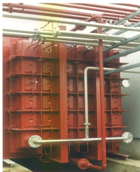
Viste anteriore e posteriore autoclave da m 3 51 in AISI 304 Front and rear views of m 3 51 autoclave in AISI 304.
