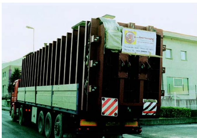
Viste anteriore e posteriore autoclave da m 3 51 in AISI 304 Front and rear views of m 3 51 autoclave in AISI 304.
