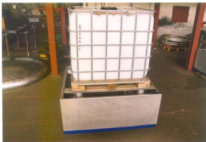
Vista laterale bonza di contenimento per spostamento liquidi e vasca porta-contenitori Lateral view of tar-laying for the containment and handling of liquids and container-holder tank.
