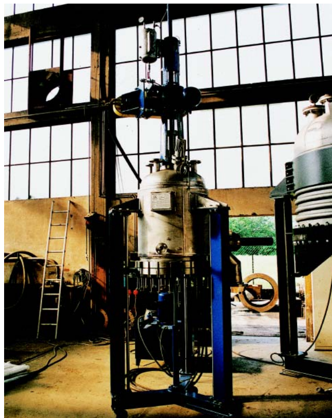
Filtro pressa DN 600 in AISI 316 collaudato secondo 97/23/CE“PED” Press filter DN 600 in AISI 316, tested according 97/23/CE“PED”
