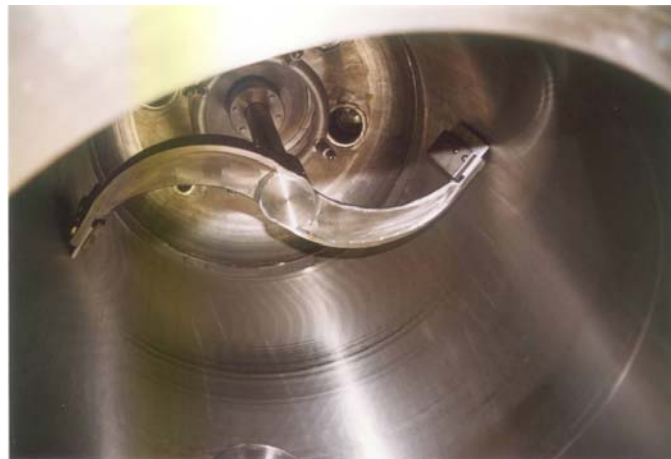
Particolari lanterna e vista interna filtro pressa DN 600 Particular lantern and interior view of press filter DN 600
