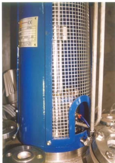
Particolari lanterna e vista interna filtro pressa DN 600 Particular lantern and interior view of press filter DN 600
