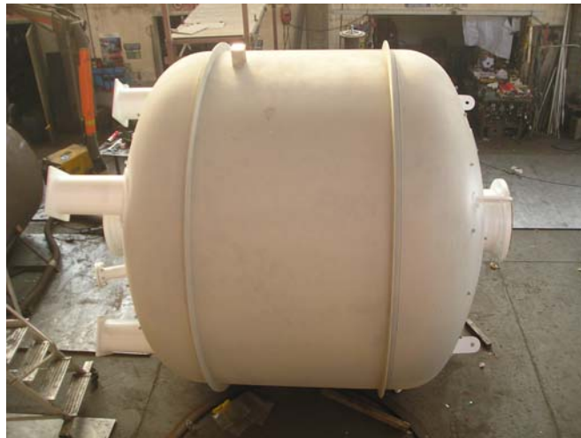
Barili prepurificatori aria/azoto DN 3200 da 22000 L in P355 NH (UNI EN 10028/3) costruiti secondo normativa 'PED' 97/23/CE e codice di calcolo VSR 22000 L DN 3200 air/nitrogen pre-purifier barrels in P355 NH (UNI EN 10028/3) built according to norm 'PED' 97/23/CE and design code VSR
