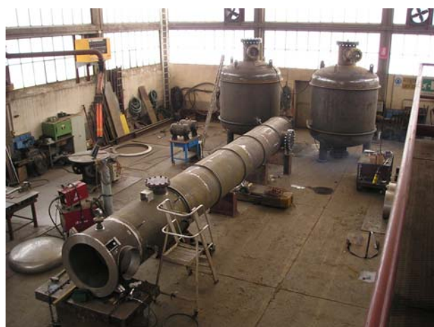
Torre di raffreddamento azoto-acqua DN1000 H9000 in P355 NH (UNI EN 10028/3) costruita secondo normativa 'PED' 97/23/CE e codice di calcolo AD2000 DN1000 H9000 nitrogen-water cooling tower in P355 NH (UNI EN 10028/3) built according to norm 'PED' 97/23/CE and design code AD2000
