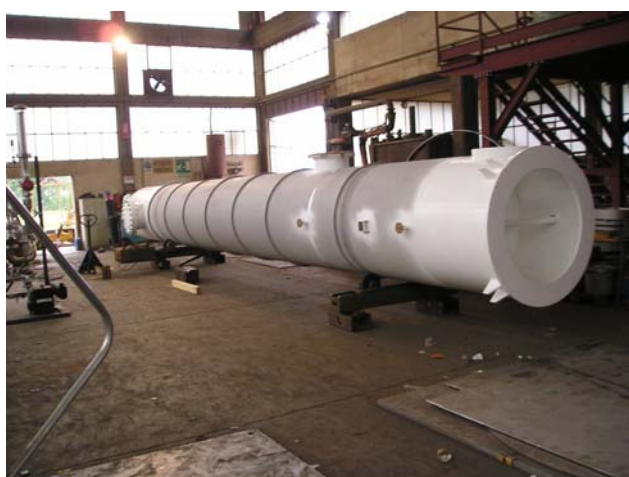
Torre di raffreddamento azoto-acqua DN 1300 H11400 in P355 NH (UNI EN 10028/3) costruita secondo normativa 'PED' 97/23/CE e codice di calcolo VSR DN 1300 H11400 nitrogen-water cooling tower in P355 NH (UNI EN 10028/3) built according to norm 'PED' 97/23/CE and design code VSR
