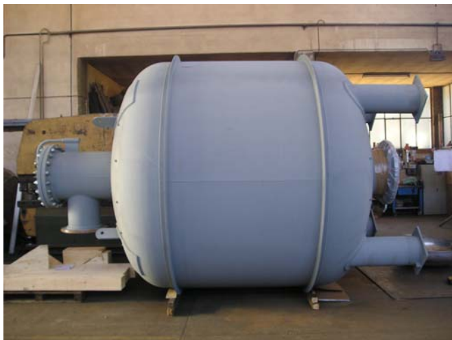
Barili prepurificatori aria/azoto DN 2800 da 16000 L in ASTM A 516 Gr.70 costruiti secondo ASME VIII Div.1 16000 L DN 2800 air/nitrogen pre-purifier barrels in ASTM A 516 Gr.70 built according to ASME VIII Div.1
