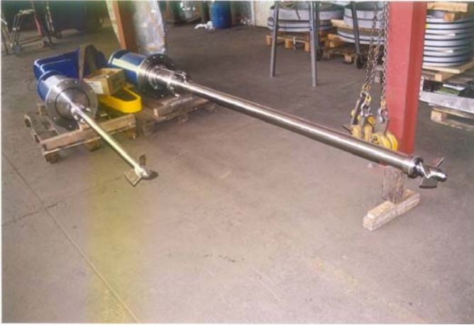
Agitatori e vista interna mescolatore per paste da L 10000 in AISI 316 Mixers and interior view of mixer for pulps, L 10000, in AISI 316.
