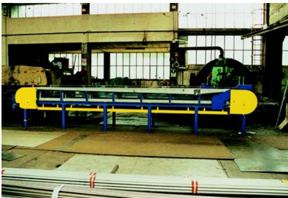
Nastro raffreddatore 1000x8000 con raschiatore e rullo raffreddato Cooling belt 1000x8000 with scraper and cooled roller
