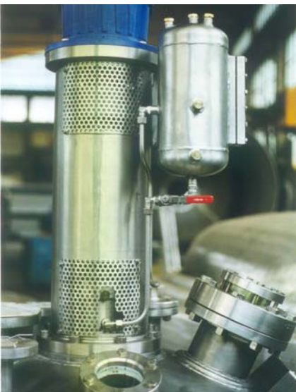
Particolari interno e lanterna reattore da L 750 in AISI 316L Interior detail and reactor's lantern, L 750, in AISI 316L
