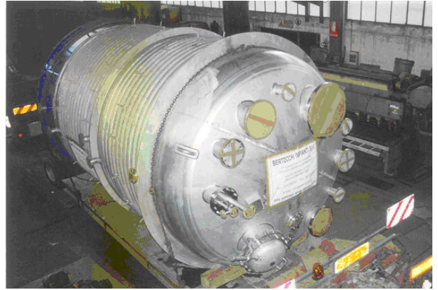
Reattore da m 3 30 in AISI 316 in accordo a dir. 97/23/CE “PED” Reactor of m 3 30, in AISI 316, in compliance with directive 97/23/CE “PED”
