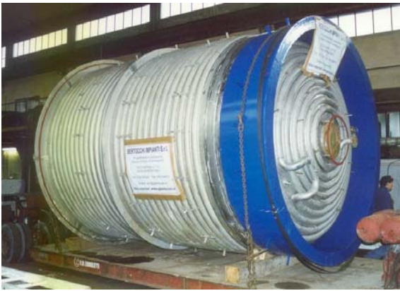
Reattore da m 3 30 in AISI 316 in accordo a dir. 97/23/CE “PED” Reactor of m 3 30, in AISI 316, in compliance with directive 97/23/CE “PED”
