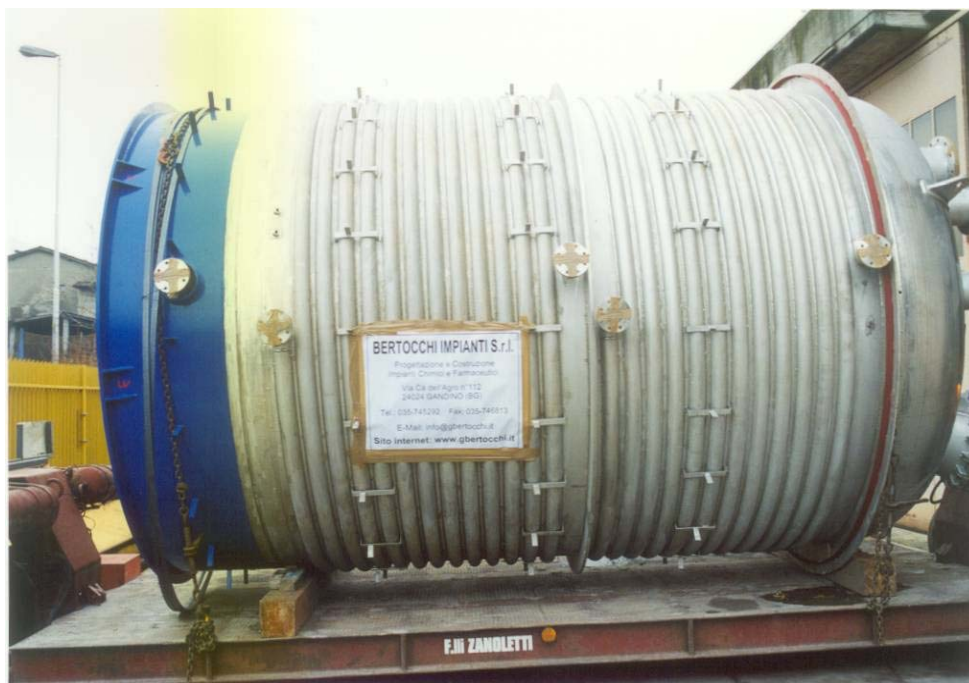
Reattore da m 3 30 in AISI 316 in accordo a dir. 97/23/CE "PED" Reactor of m 3 30, in AISI 316, in compliance with directive 97/23/CE "PED"
