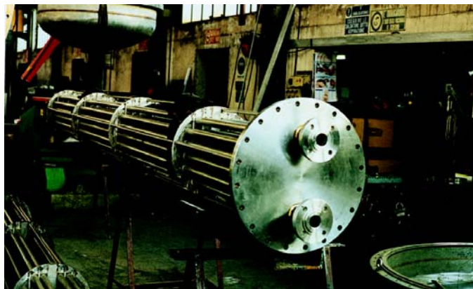
Fascio tubiero per riscaldatore a vapore in AISI 316 collaudato 50 bar Tube bundle for steam heater in AISI 316, tested at 50 bar
